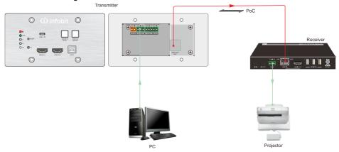
3) If the switcher needs to be controlled by receiver end, the control device (e.g. PC) can be connected to the RS232 port of the receiver, the connection diagram shown as below:
