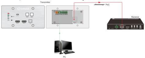
2) If the far-end third-party device (e.g. projector) need be controlled by PC, please connect the third party device (e.g. projector) to the RS232 port of receiver. The connection diagram shown as below:
