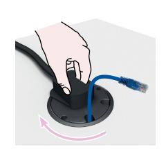
Rotate plug clockwise to reattach.
